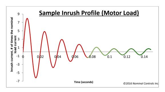
The effect of inductive reactance, power grid variables and other tolerances also need to be considered while choosing the SSR's current rating. However a lower SSR current rating may be permitted if the load's start-up current follows a lower and gradual increasing inrush current profile such as motor soft-start. As a rule of thumb, choose SSR rated 50% of the expected peak inrush current. The following table shows the respective inrush current profiles of different types of loads:
